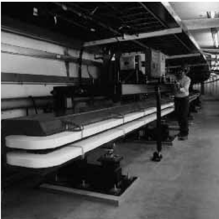
Typical magnets for the low-energy ring (above) and high-energy ring (below) in PEP-II.
