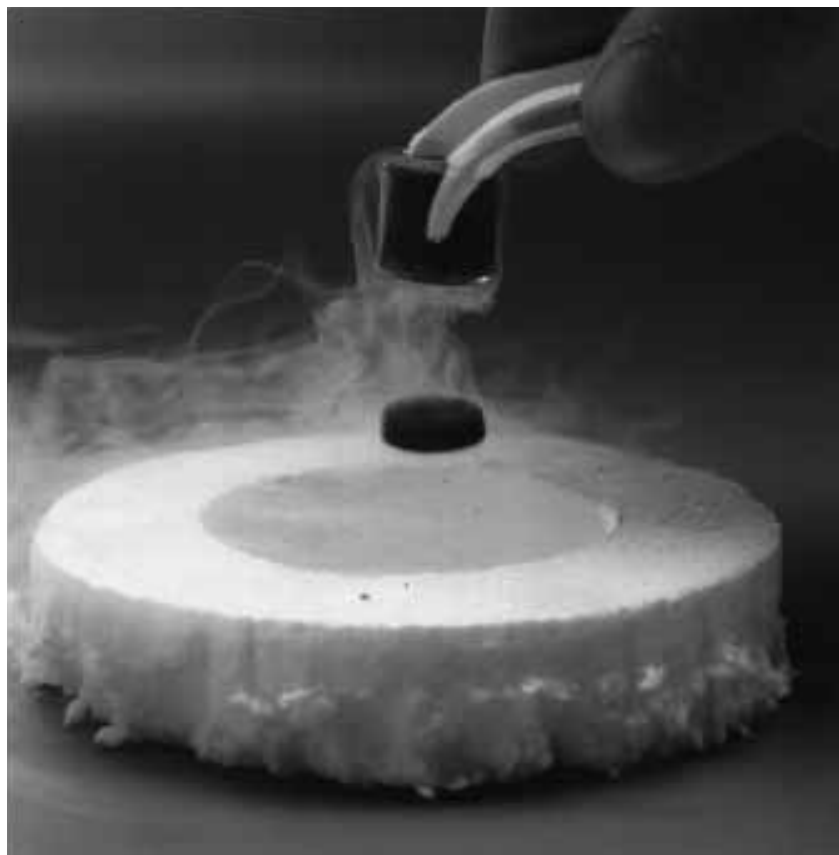
A high- T_c ceramic superconductor levitates a magnet. (Courtesy Science Kit & Boreal Laboratories)
