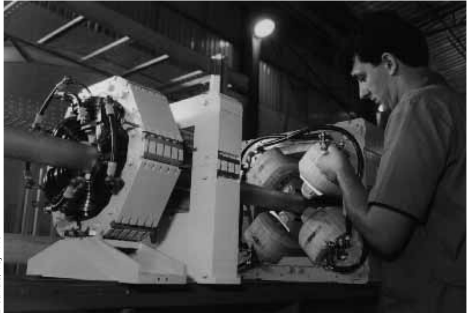
Putting the finishing touches on a quadrupole magnet for the storage ring.
