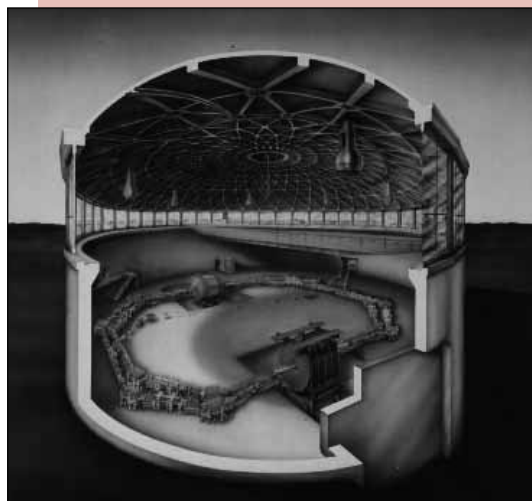
An artist's view of the two rings of the DAΦNE complex showing the magnet layout and the two detectors, KLOE for particle physics on the right and FINUDA for nuclear physics on the left.
