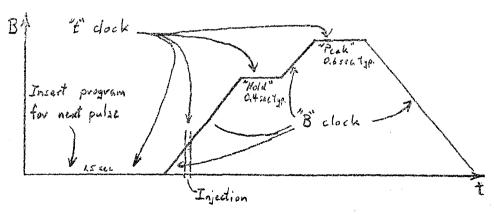
By using two "clocks," one counting a megacycle oscillator and the other counting (integrating) the output of a voltage-frequency converter looking at dB/dt from a sampling loop, Lewis can program any shape pulse (with several "holds" if desired) and can program successive pulses differently.
