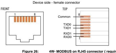
4W- MODBUS on RJ45 connector (required pin-out)
