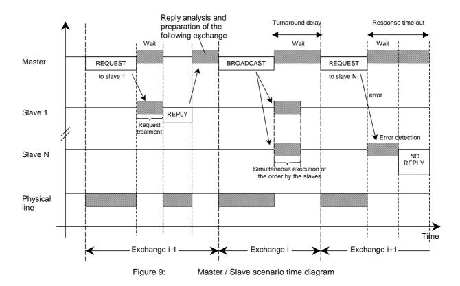
This following figure shows the time diagram of 3 typical scenarios of Master / Slave communications.
