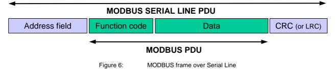
• On MODBUS Serial Line, the Address field only contains the <u>slave address</u>.
