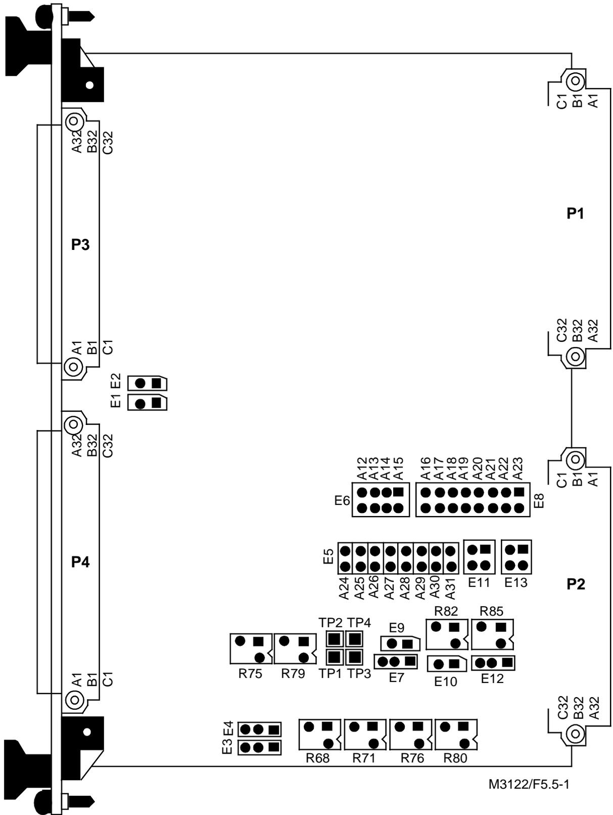
Figure 5.5-1. Locations of Test Points and Adjustments
