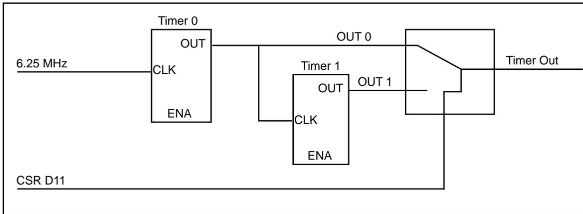
Figure 4.4.6-1. VMIVME-3122 Timer Functional Block Diagram
