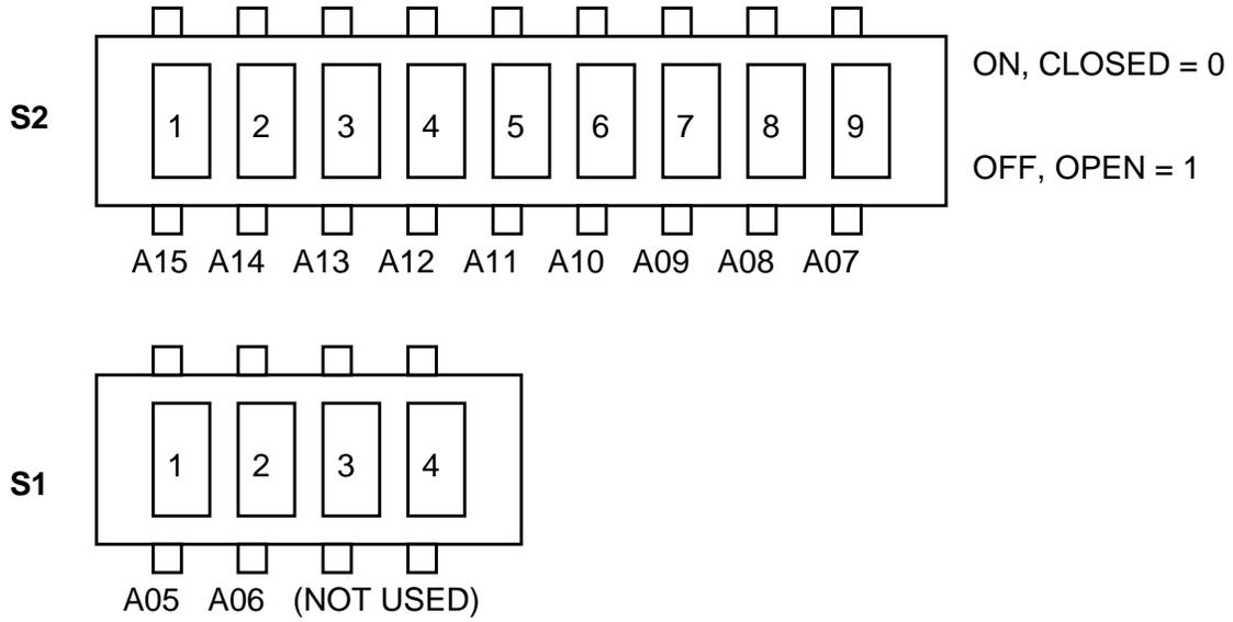
For the VMIVME-4100 to respond to a base address of  $(FFFF00)_{16}$  the S1 and S2 switches would be set accordingly.
