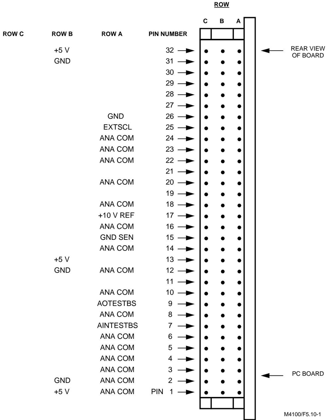
Figure 5.10-1. P2 Connector - Pin Assignments
