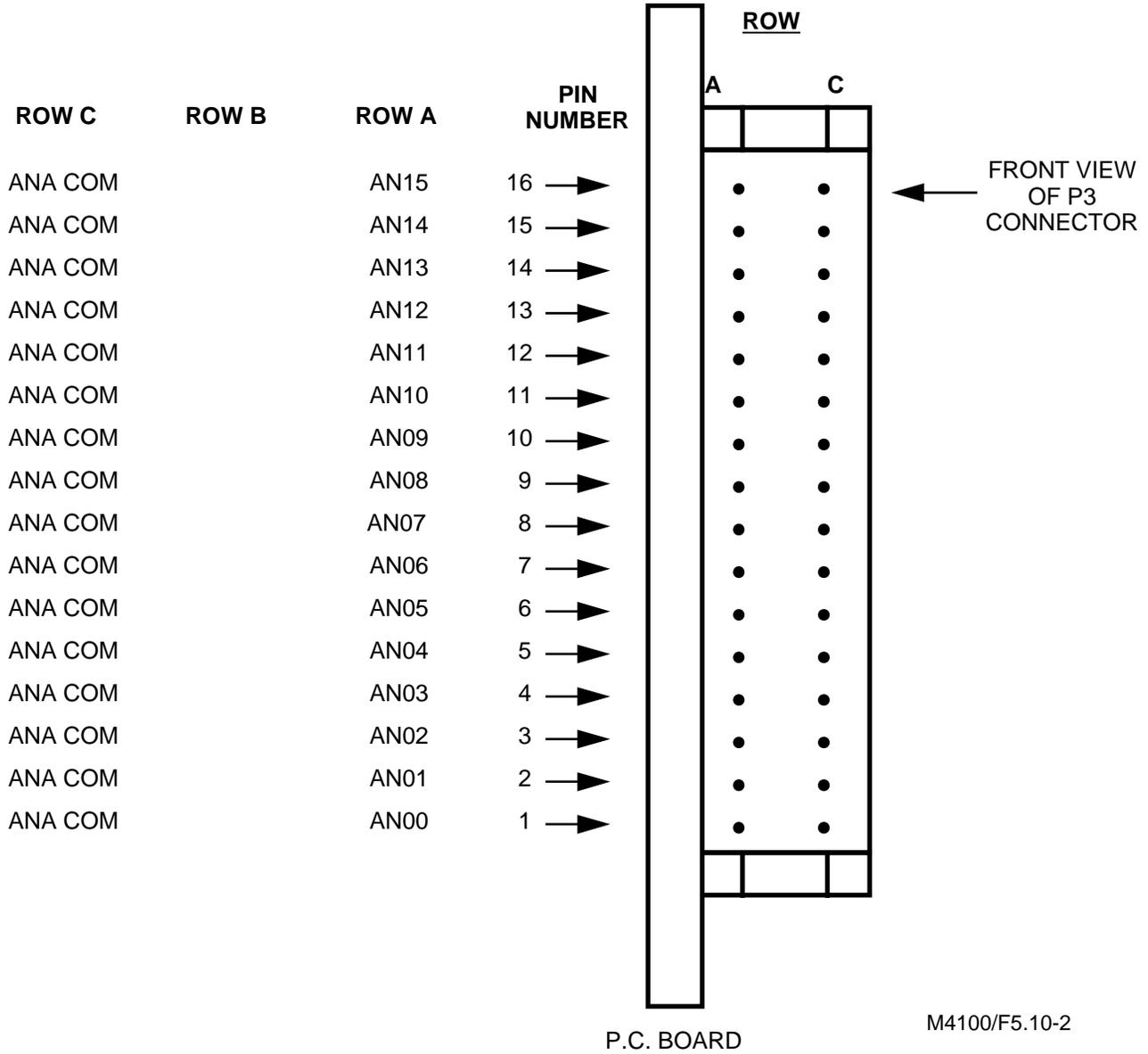
Figure 5.10-2. P3 Connector - Pin Assignments
