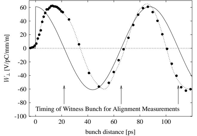
**Figure 6:** Transverse wakefield inferred from the deflection of the witness bunch for large drive beam offsets as a function of time (dots), a scaled prediction (dotted line) and the expected variation of the fundamental mode component (solid line, arb. units). For alignment measurements the wakefield curve was sampled at the indicated three points.
