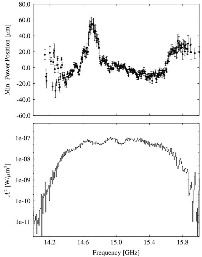
**Figure 4:** Minimum power positions  $y^{\min}$  (upper plot) and fit parameter  $A^2$  from Eq. (1) (lower plot) as a function of frequency for a beam position scan in the vertical plane. Note the zero position in the upper plot is arbitrarily defined.
