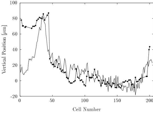
**Figure 5:** Cell to cell alignment, inferred from the minimum power position measurement (dots), compared to a mechanical straightness measurement (solid line).
