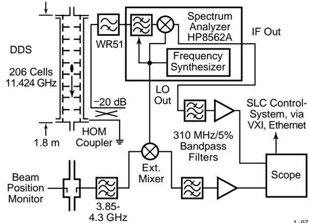
**Figure 2:** Electronic setup for the detection and processing of the DDS manifold signals.
