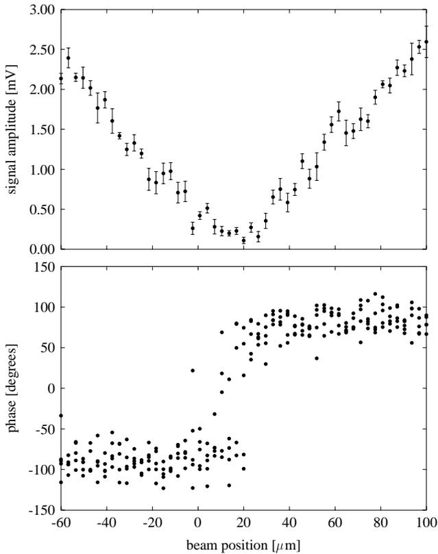
**Figure 7:** Amplitude and phase of the dipole mode signal at a frequency of 14.9675 GHz as a function of the vertical beam position. For each beam position 5 pulses have been measured. The vertical beam jitter amounts to 15  $\mu\text{m}$  rms.
