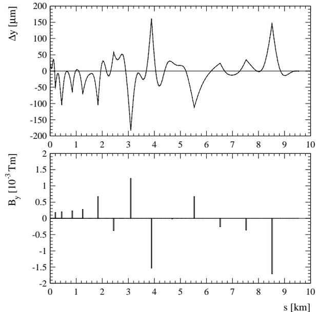
Figure 1: Example of the beam-based alignment algorithm with perfect BPM's and RF-BPM's. The initial random quadrupole misalignment was  $100\ \mu\text{m}$  rms. The alignment is done in 14 sections and 15 iterations. At the end of each section a dipole corrector is used to launch the beam into the next section. The upper plot shows the misalignment  $\Delta y$  of quadrupoles, RF-structures and BPM's after alignment. The lower plot shows the integrated fields of the dipole correctors.
