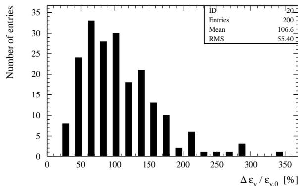
Figure 2: Histogram of vertical emittance growth  $\Delta\epsilon_y/\epsilon_{y,0}$  for 200 different error distributions. The average emittance growth is  $106.6\% \pm 3.9\%$ . Note the exponential distribution for large emittance dilutions.
