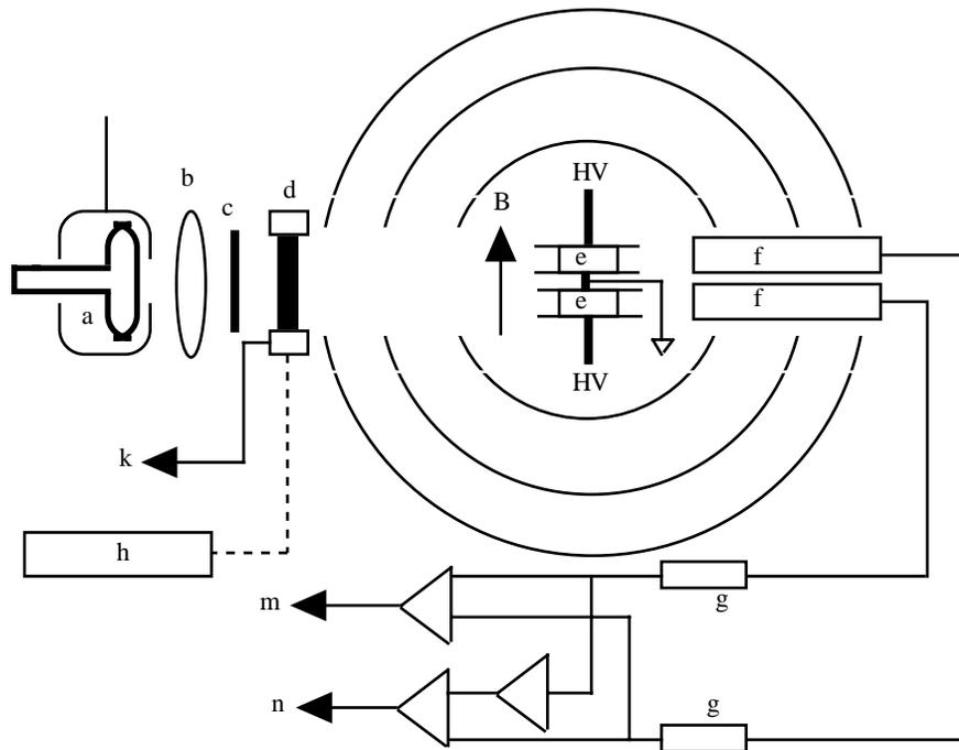
Fig. 7. Schematic diagram of Seattle  $^{199}\text{Hg}$  EDM experiment. a:  $^{204}\text{Hg}$  lamp; b: lens; c: linear polarizer; d: quarter-wave plate; e: optical pumping cells; f: optical detectors; g: phase sensitive detectors; h: stepping motor; k: phase sensitive detector reference; m: magnetic field and gradient correction signals.
