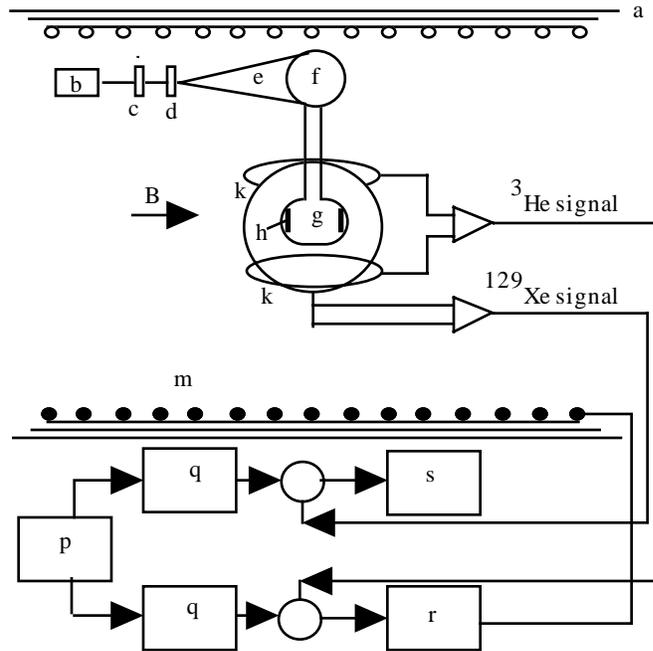
Fig. 8. Schematic diagram of Harvard/Smithsonian-Michigan  $^{129}\text{Xe}$  EDM experiment. a: nested magnetic shields; b: 795 nm light source; c: quarter wave plate; d: beam expander; e: light beam; f: pump bulb; ( $T=120\text{ C}$ ); g: maser bulb; ( $T=40\text{ C}$ ); h: electric field plates; h: pickup coils; m: main solenoid; p: LORAN reference; q: frequency synthesizers; r: phase-sensitive current source; s: A/D converter.
