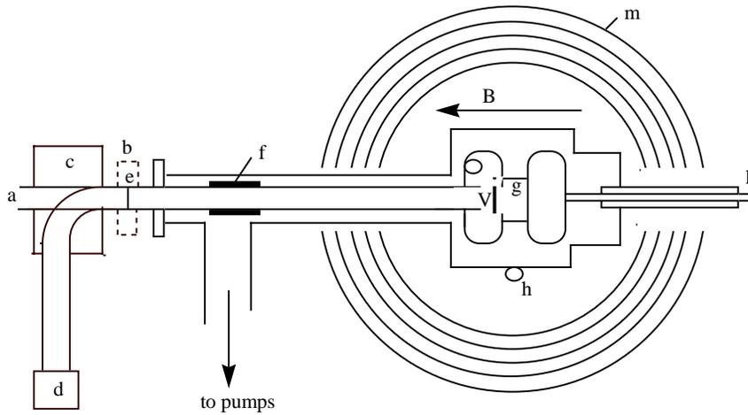
Fig. 4. Schematic diagram of 1990 I.L.L. neutron EDM expt. a:UCN entrance; b: magnet; c: guide changer; d: UCN detector; e: polarizing foil; f: flip coil; g: storage chamber; v: neutron valve; k: rubidium magnetometer; m: 5 layer magnetic shield; p: HV feedthrough.
