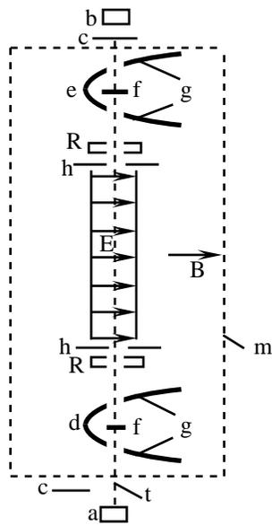
Fig. 9. Schematic diagram of 1994 Berkeley  $^{205}\text{Tl}$  electron EDM experiment. a: up-beam oven; b: down-beam oven; c: automatic beam stops; d: state selector region; e: analyzer region; f: 378 nm laser beams ( $\perp$  to page); g: 535 nm fluorescence; h: collimating slits; E: 107 kV/cm electric field; B: static magnetic field; m: 4-layer magnetic shield; R: radio frequency field regions; t: Tl atomic beam.
