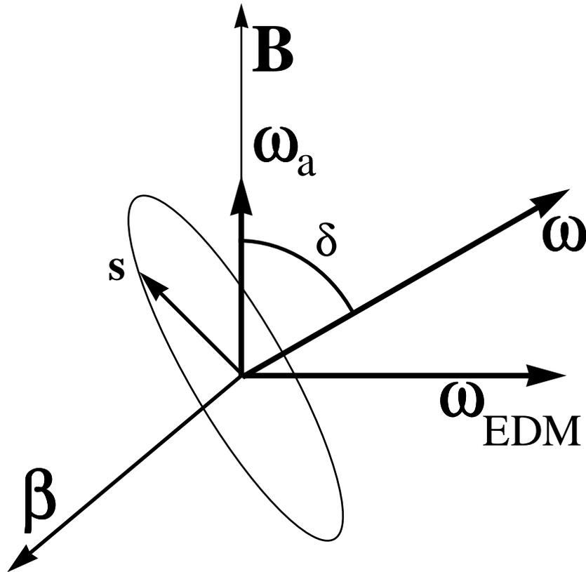
Fig. 11. Schematic diagram (not to scale) of relevant vectors in muon spin-precession experiment, as described by the BMT equation.  $\beta$ : muon velocity;  $\mathbf{B}$ : applied magnetic field;  $\omega_a$ : ang. vel. of precession due to  $g-2$ ;  $\omega_{EDM}$ : ang vel of precession due to EDM;  $\omega$ : resultant;  $\delta$ : angle between  $\omega$  and  $\mathbf{B}$ ;  $\mathbf{s}$ : muon spin vector, which precesses about  $\omega$ .
