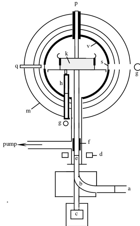
Fig. 5. Schematic diagram of the current I.L.L. neutron EDM experiment. a: UCN source; b: neutron guide change-over; c: UCN detector; d: magnet; e: polarizing foil; f: flip coil; g: Hg UV lamps; h: cell for pre-polarization of Hg atoms; k: storage volume; m: 4-layer magnetic shield; p: HV lead; q: UV light detector; v: vacuum wall; s: optical windows.
