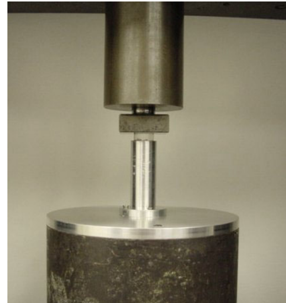
Shear Strength Test Set-up
