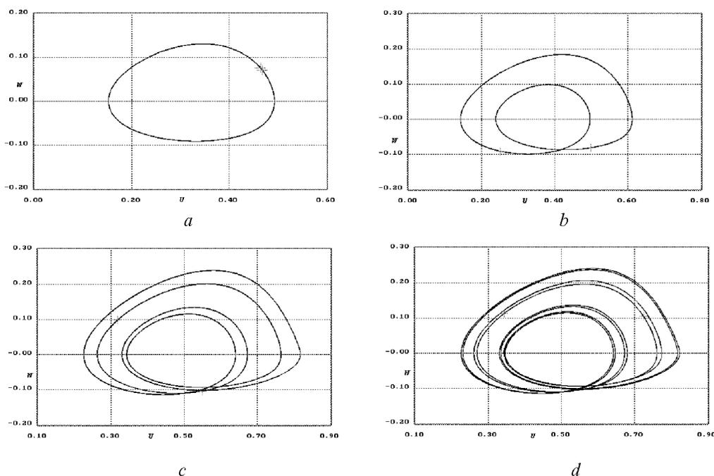
Fig.2. Period doubling bifurcation in system (4).  $\beta = -0.8$ ,  $\xi = -1.25$ ,  $\kappa = 0.05$ ,  $\gamma = \kappa\xi/D$ . For case *a*:  $D = \sqrt{3}$ ; for case *b*:  $D = \sqrt{3.2}$ ; for case *c*:  $D = \sqrt{3.7}$ ; for case *d*:  $D = \sqrt{3.71}$
