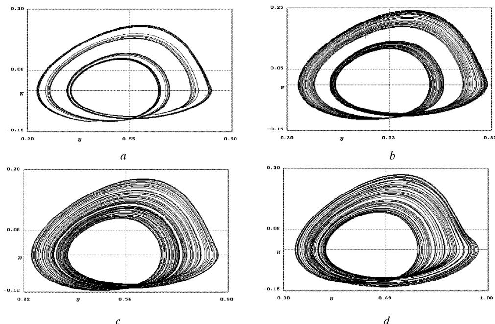
Fig.3. Patterns of chaotic trajectories of system (14).  $\beta = -0.8$ ,  $\xi = -1.25$ ,  $\kappa = 0.05$ ,  $\gamma = \kappa\xi/D$ . For case a:  $D = \sqrt{3.73}$ ; for case —it b:  $D = \sqrt{3.75}$ ; for case c:  $D = \sqrt{3.83}$ ; for case d:  $D = \sqrt{4.299}$
