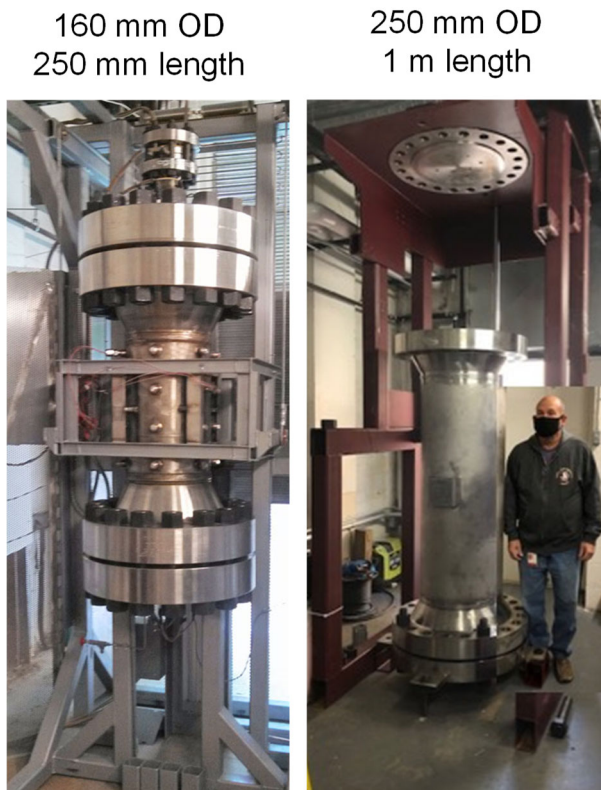
Figure 6: Reaction furnaces for Bi-2212 test coils operating at 50 bar pressure through the reaction sequences like that shown in Figure 5. Dimensions reflect the internal diameter and length of the uniform temperature zone. The larger furnace at right is being commissioned in 2022.
