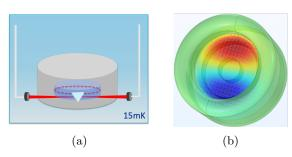
FIG. 6: (a) Block diagram of a microwave-optical bulk transduction device; (b) microwave design, dipole mode excited in the cavity with maximum electric field on the edge of the crystal.
