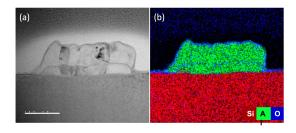
FIG. 3: (a) Bright -field transmission electron microscopy image and (b) corresponding Energy Dispersive X-ray Spectroscopy (EDS) elemental mapping of a Josephson junction made by aluminum metals with ultra-thin aluminum oxide in between.
