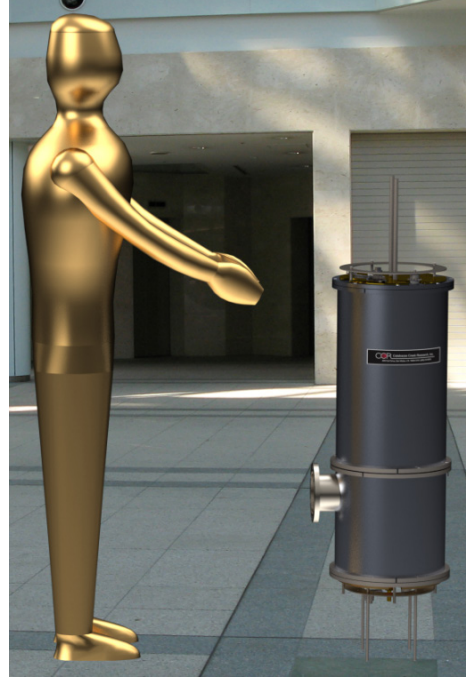
Figure 11. Image of 200 kW, 350 MHz multiple beam triode RF source model
