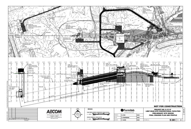
Figure 10: Elevation of the LBNF near site, showing the target hall, decay pipe, and the near detector hall. The boundary between soil and rock is shown. The vertical scale is expanded by a factor of two with respect to the horizontal scale. Both scales are measured in feet.
