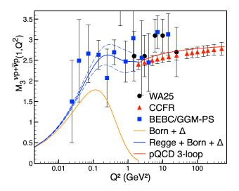
Figure 5: World data on the first Nachtmann moment  $M_3^{\bar{\nu}p+\nu p}(1,Q^2)$  of the CC inclusive structure function  $F_3$  as a function of  $Q^2$  along with theoretical curves (see text for explanation).
