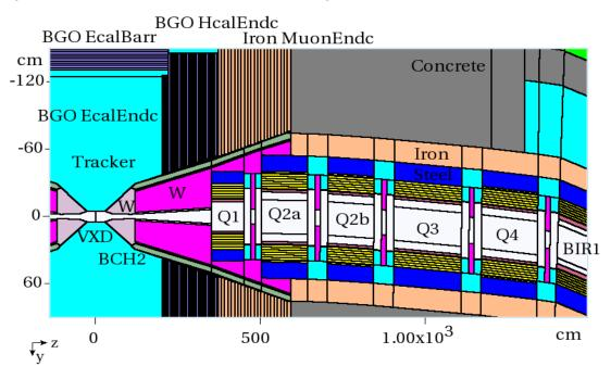
Figure 6: MDI MARS15 model with tungsten nozzles on each side of IP, tungsten masks in interconnect regions and tungsten liners inside each magnet [3, 5].
