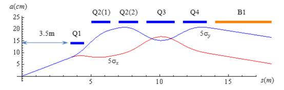
Figure 1: Higgs factory IR quadrupoles aperture and 5s beam envelopes for  $\beta^* = 2.5$  cm.
