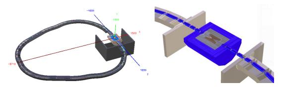
Figure 5: 3D MARS15 models of the HF MC (left) and MDI with SiD-like detector (right).
