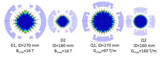
Figure 3: Coil cross-sections and parameters of HF SR dipoles and quadrupoles.
