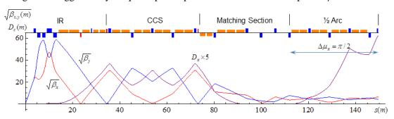
Figure 2: Layout and optics functions in half ring of the Higgs factory.
