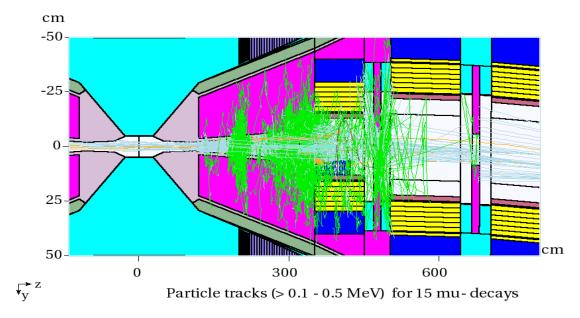
Figure 7: Visualization of the Higgs Factory machine and detector protection system efficiency for particle tracks arriving at the Machine-Detector interface from the right side [5].
