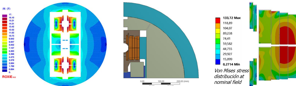
Fig. 3: Design studies performed for 16 T common coil dipole for FCC by CIMET.
