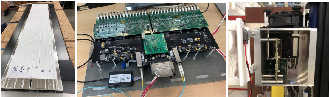
FIG. 3. Left: A scintillator layer of the HCal prototype composed of two sets of four bars each. Center: Prototype of LDMX HCal custom readout electronics which digitizes 256 SiPM signals using the HGCROCv2. Digitized signals are aggregated on an FPGA mezzanine and transmitted optically to a central ATCA-based DAQ system. Right: the prototype TS module. Scintillators are read out by 12 SiPMs, whose signals are digitized by a QIE11 hosted on a readout board, shown vertically in the aluminum housing. Data is transmitted optically over a pair of fibers to the trigger and DAQ system.
