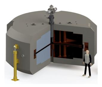
Figure 4.6: 3/4 cut view of a CAD rendering of the IsoDAR cyclotron with RFQ direct injection.
