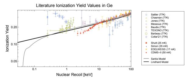
Figure 1: Ionization yield measurements in Ge (right) below 100 keV. The solid and dashed lines represent the predictions of the Lindhard and Sarkis models [10, 11]
