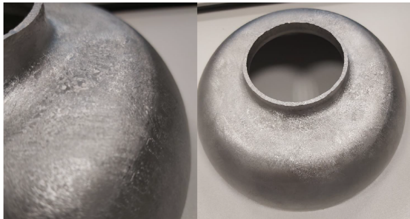
Fig. 11: Picture of a cavity with RRR~100 MG Nb after deep drawing (Courtesy of Research Instruments, GmbH).
