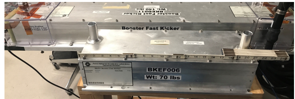
Figure 7: An example of a short kicker for PAR extraction is the Booster style short kicker.
