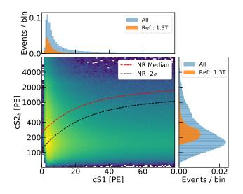
FIG. 35. Illustration of the accidental coincidence background distribution from XENON1T in cS1 and log10(cS2b), with projections on each axis showing the expected distribution within the entire analysis space (blue), and in the reference region for 1.3 tonne fiducial volume. The reference region lies between the nuclear recoil median and  $-2\sigma$  quantile lines, marked by red and black lines, respectively. Figure from Ref. [1061].
