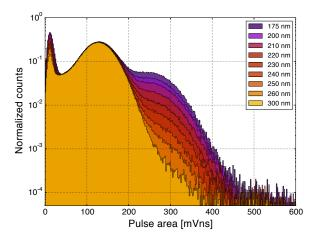
FIG. 16. Superposition of single photon pulse area spectra of a R11410 PMT for different wavelengths. Each spectrum is normalized by the integral in the region between 50–120 mV ns in order to show the effect more clearly. Figure from Ref. [475].
