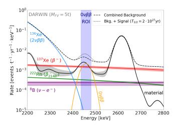
FIG. 22. Predicted background spectrum around the  $0\nu\beta\beta$ energy region of interest (ROI) for a proposed next-generation dark matter experiment. Rates are averaged over a fiducial volume (FV) containing 5000 kg of liquid xenon with natural isotopic abundance. Bands indicate  $\pm 1\sigma$  uncertainties. The orange line represents a hypothetical signal corresponding to  $T_{1/2} = 2 \times 10^{27}$  years. Figure from Ref. [663].
