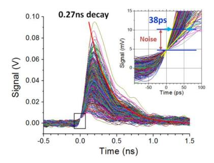
Figure 5: Scope traces of events from  $\text{Am}^{241}$  events. Recorded pulses showing 100 ps rise time, 270 ps decay time, and 38 ps time resolution with average collected charge of  $1.5 \times 10^5$  electrons. Adapted from Ref. [40].
