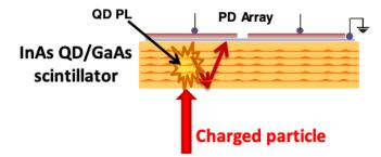
Figure 4: A schematic drawing of the proposed tracking sensor. A charged particle enters the GaAs scintillator, producing electron-hole pairs. The electrons are then quickly trapped by the positively charged InAs quantum dots (QDs). The QDs undergo photoluminescence (PL) and emit photons that travel through the medium. The emitted photons are collected by a photodiode (PD) array.
