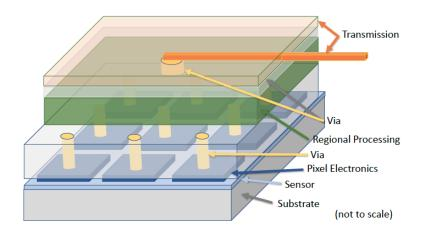
Figure 3: The conceptual stack-up of a monolithic thin film detector that incorporates support structure, sensor, pixel electronics, regional processing electronics, and power/data transmission. Potentially, no other structures would be needed in the detector volume.
