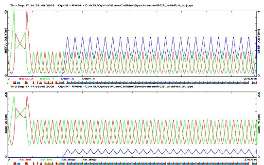
**Figure 2**: The beta-functions and dispersion (top) and the beam envelopes (bottom) for a half of the ring (the injection & extraction straight and downstream arc.) The beam envelopes are shown at injection for  $\varepsilon_n$ =40 mm mrad,  $E_k = 2$  GeV,  $\Delta p/p = 5 \times 10^{-3}$ .
