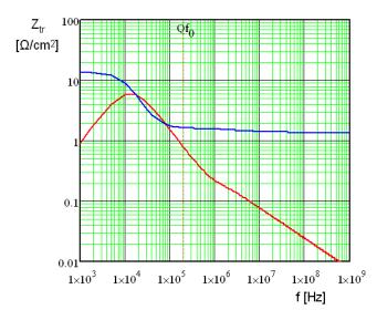
**Figure 3**: The dependence of real (red) and imaginary (blue) parts of transverse impedance per unit length on the frequency for round stainless steel vacuum chamber: radius of 22 mm, wall thickness of 0.7 mm, and the beam energy 2 GeV.
