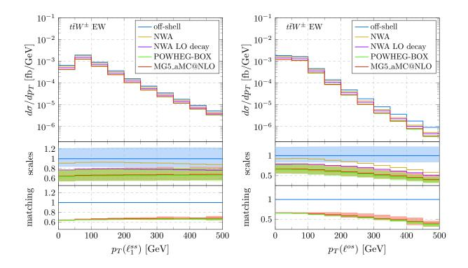
FIG. 6. Differential cross section distribution in the  $3\ell$  fiducial region as a function of the transverse momentum of the hardest same-sign lepton  $\ell_1^{ss}$  (l.h.s.) and the opposite-sign lepton  $\ell^{os}$  (r.h.s) for the  $pp \rightarrow t\bar{t}W^{\pm}$  EW process. The uncertainty bands correspond to independent variations of the renormalization and factorization scales (middle panel) and of the matching parameters (bottom panel).
