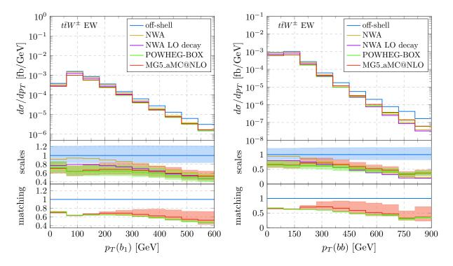
FIG. 5. Differential cross section distribution in the  $3\ell$  fiducial region as a function of the transverse momentum of the hardest b jet (l.h.s.) and of the system of the two hardest b jets (r.h.s) for the  $pp \rightarrow t\bar{t}W^{\pm}$  EW process. The uncertainty bands correspond to independent variations of the renormalization and factorization scales (middle panel) and of the matching parameters (bottom panel).
