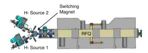
FIG. 12. Two PIP-II ion sources, LEBT, and RFQ
