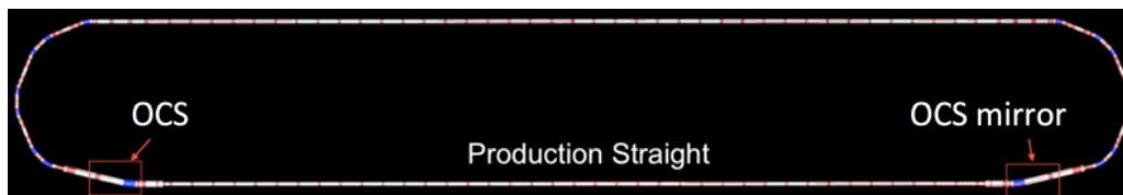
FIG. 3: Racetrack ring layout. Pions are injected into the ring at the Orbit Combination Section (OCS). Similarly, extraction of pions and muons at the end of the production straight is done using a mirror image of the OCS.
