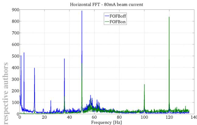
Figure 3: Horizontal FFT of beam position when FOFB was ON and OFF. Trim coil components are identified at 1.2, 3.6, 12, 36 and 120 Hz.
