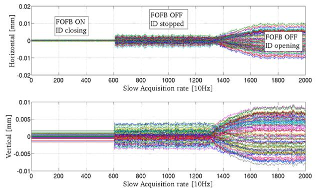
Figure 5: BPMs position when closing/opening the ID.
