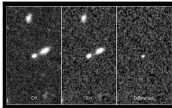
Transient Detection with Image Differencing (CANDELS; <http://www.spacetelescope.org/images/heic1306d/>)
