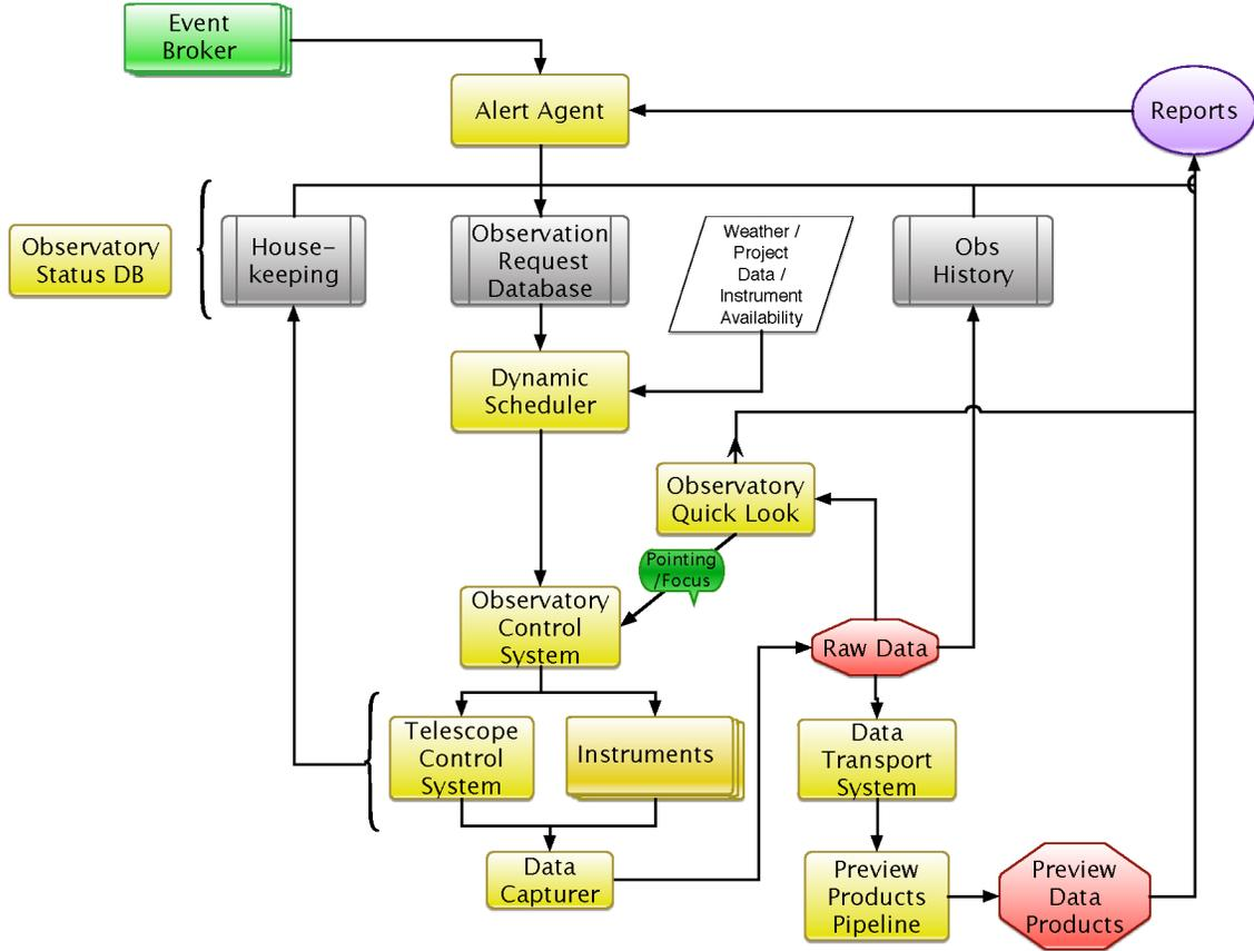
Figure 2: Flow chart of the CCAT software system from the perspective of processing transient alerts.
