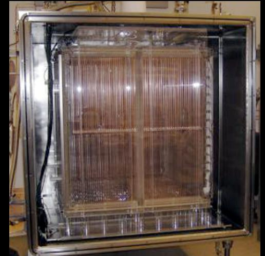
**NEWAGE:** in Kamioka,  $\mu$ -pattern gas detector readout,  $\text{CF}_4$  gas, *first* directional dark matter limit!
