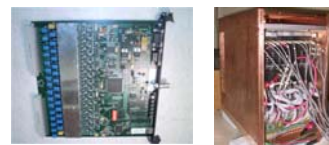
150 ionization channels and 74 LAAPD channels are sampled at 1 MHz by 12-bit ADCs.
