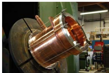
The TPC is housed in a thin-walled low-activity copper vessel. The parts have been machined under 7 m.w.e. concrete to protect them from cosmogenic activation and are electron beam welded together.
