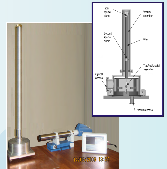
Figure 1 A photograph of the assembled torsion balance together its blueprint (inset). The laser autocollimator together with the dedicated computer (lower middle and right) are illustrated too.
