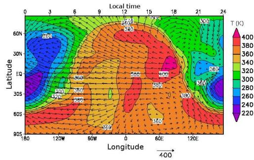
Figure 2: Temperatures (color contours) and winds (arrows) in a constant pressure layer in the upper thermosphere ( $P \approx 10^{-9}$  Pa) derived from the LMD-MGCM for perihelium conditions.
