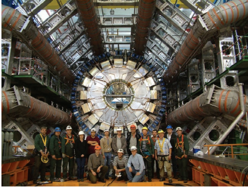
Figure 2, the ATLAS barrel calorimeter position inside the toroid magnets on the interaction point.
