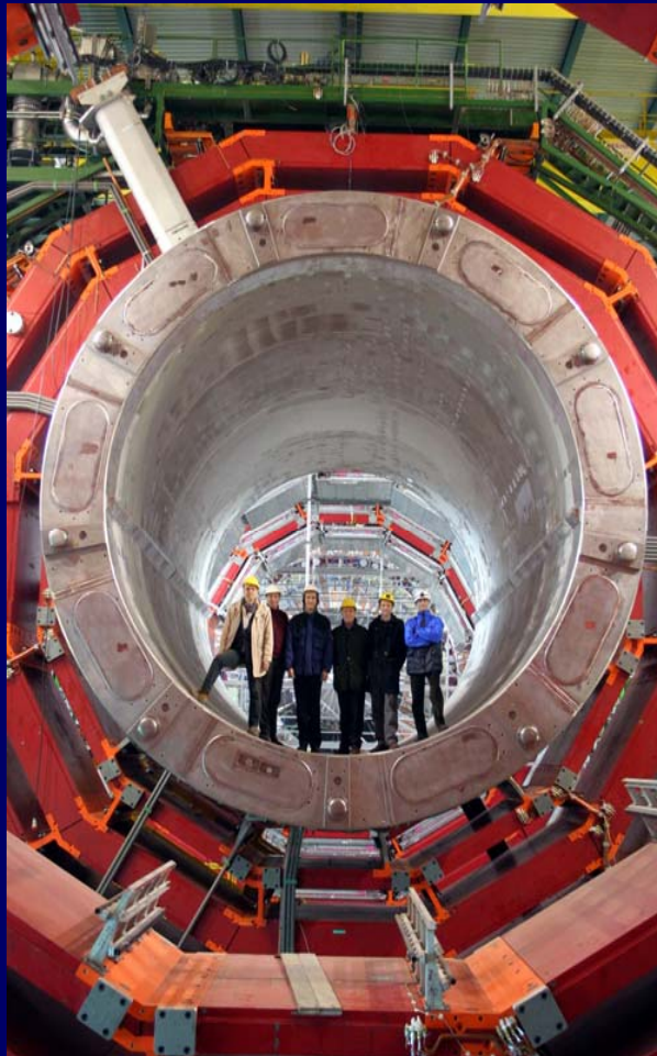
Vacuum Tank welded (Nov-Jan)
