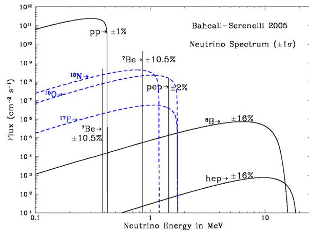
Figure 2: Solar neutrino energy spectra. Figure from Reference Bahcall et al. [2005].
