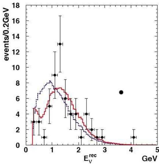
Figure 6: Energy spectrum of single ring events in SuperK for the K2K experiment. Solid line is the best fit spectrum with oscillations and the dashed line is the best fit line without oscillations. Both histograms are normalized to the number of events observed. Figure taken from Reference Ahn et al. [2006].
