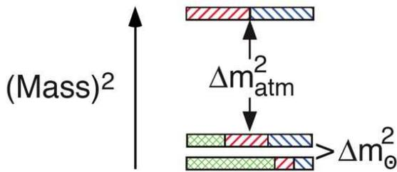
Figure 1: The ‘normal hierarchy’ of neutrino masses in a 3-generation framework which describes current experimental results with the exception of LSND. The  $\nu_e$  component of each mass state is crosshatched, the  $\nu_\mu$  component is indicated by right-leaning hatching, and the  $\nu_\tau$  component is indicated by left-leaning hatching. From Reference Eidelman et al. [2004].
