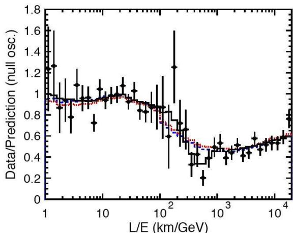
Figure 5: Ratio of the data  $L/E$  distribution to the Monte Carlo expectation for atmospheric neutrino events in the SuperKamiokande experiment. The best fit to a neutrino oscillation hypothesis is shown by a solid line, together with neutrino decay (dashed line), and neutrino decoherence (dotted line). Figure taken from Reference Ashie et al. [2004].
