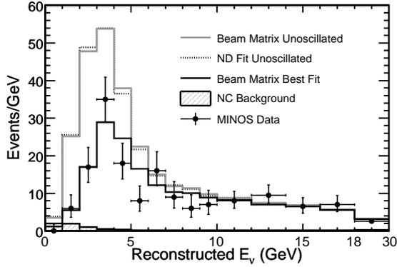
Figure 11: The MINOS Far Detector spectrum compared to the predictions for no oscillations and with a best fit oscillation model. The unoscillated prediction from two beam extrapolation methods are shown. From Reference Michael et al. [2006].
