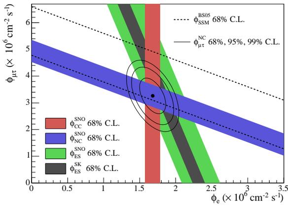
Figure 3: The flux of muon and tau neutrinos versus the flux of electron neutrinos as measured by the SNO experiment. Charged current (CC), neutral (NC) and elastic scattering (ES) results are given as bands. Dashed lines indicate the predictions for the total neutrino flux from Reference Bahcall et al. [2005]. Ovals indicate the 68, 95, and 99% CL intervals from the combined data Aharmim et al. [2005].
