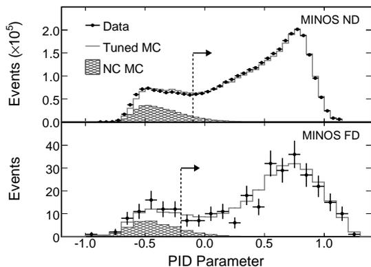
Figure 10: Data and MC predictions for the CC-like PID variable. The Near Detector is shown at the top, Far Detector the bottom. Contributions from NC events are shown by the hatched histogram. From Reference Michael et al. [2006].
