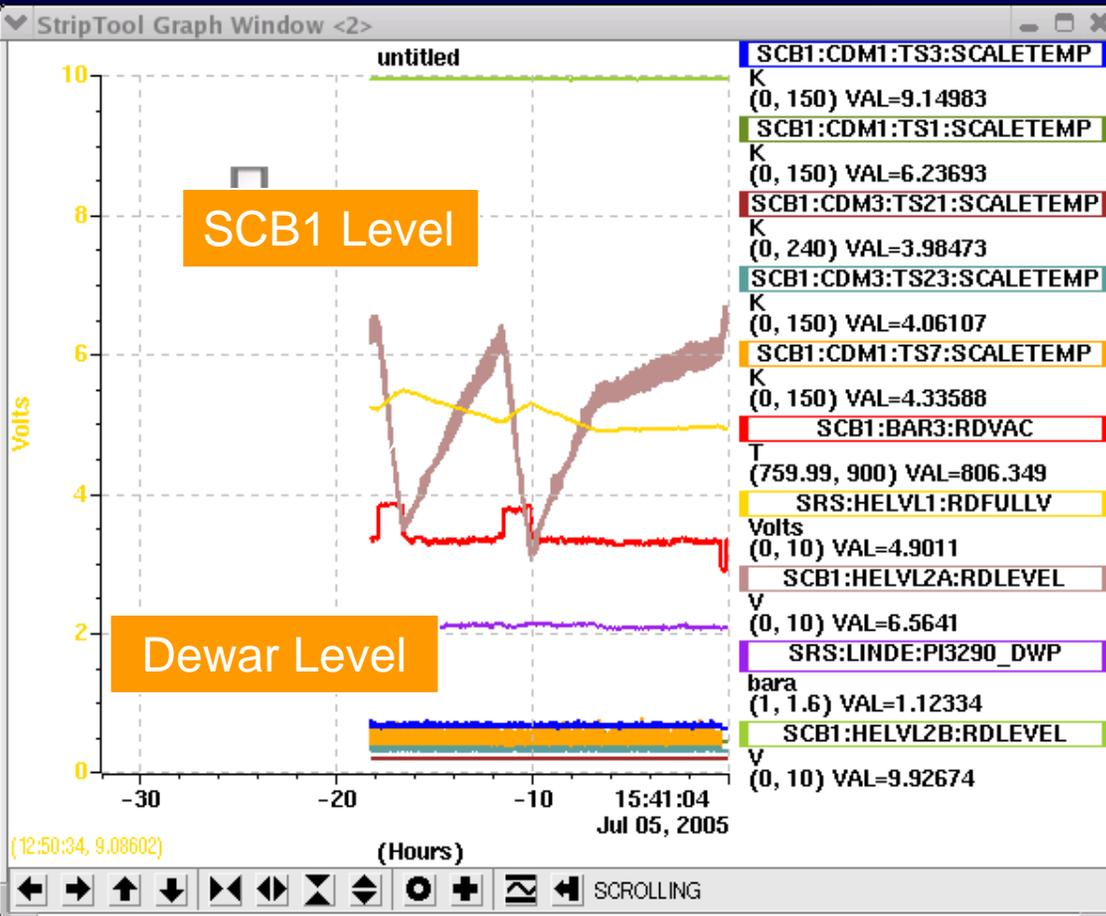
Refrigerator operated in continuous mode after an initial startup period.
