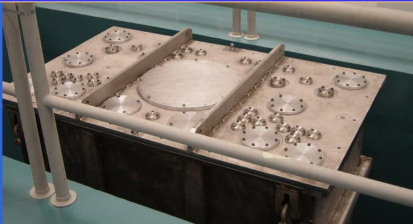
Cryomodule Vacuum Tank
