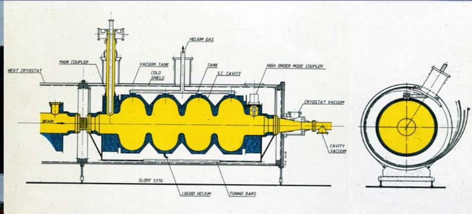
SUPERCONDUCTING CAVITY WITH ITS CRYOSTAT
