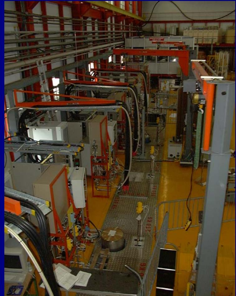
Solid polarized proton and deuteron targets. Polarized with dynamic nuclear polarization (DNP) in a 2.5 T longitudinal field generated by a s.c. solenoid and cooled to less than 1 K by a dilution refrigerator
