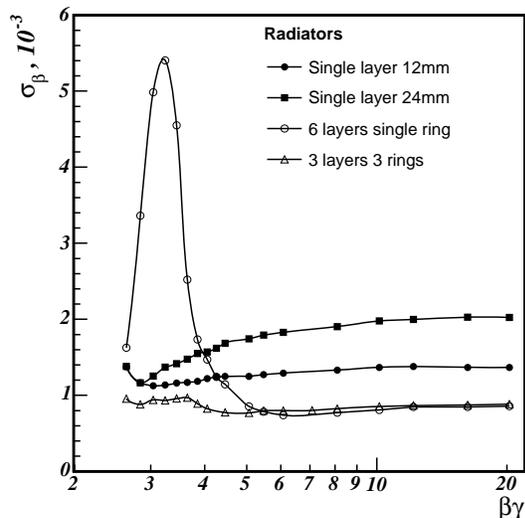
Figure 2:  $\beta$  resolution for track vs  $\beta\gamma$ , 30° particle dip angle.
