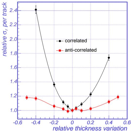
Figure 5: The dependence of the resolution from the change in the thickness of the layers.
