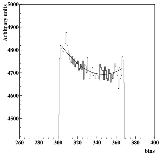
Figure 9: The longitudinal density variation in the middle of the block.
