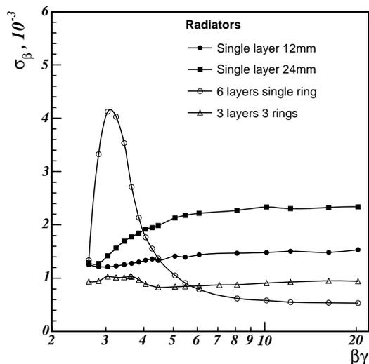
Figure 1:  $\beta$  resolution for track vs  $\beta\gamma$ . Normal particle incidence.
