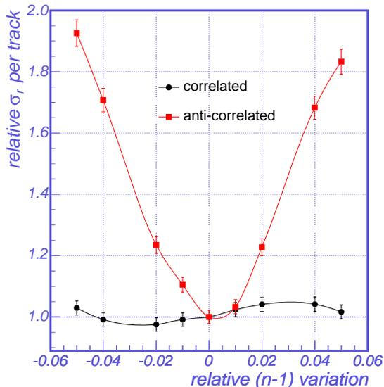
Figure 4: The dependence of the resolution vs the variation of the refractive index of the layers.
