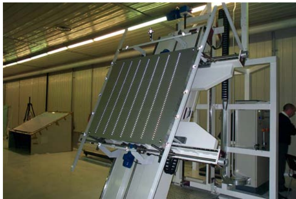
Figure 7: Workbench for testing the 40 meter panels at different elevations using photogrammetry.
