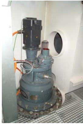
Figure 6: One of the four azimuth drive assemblies of the 40 meter radio telescope.
