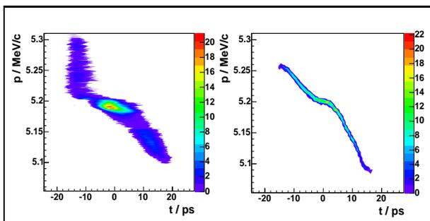
Figure 3: Measured (left) and simulated (right) longitudinal phase space. The vertical axis represents the electron beam momentum and the horizontal the temporal distribution of the bunch. Bunch charge is 1 nC.
