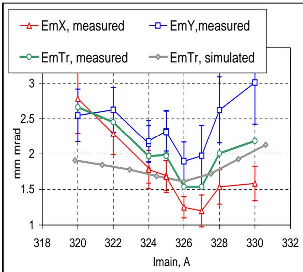
Figure 2: Normalized emittance measured at PITZ as a function of the main solenoid current. The electron beam momentum is 5.2 MeV/c, and the bunch charge 1 nC. The bucking solenoid current is optimized for each main solenoid current. Horizontal (red) and vertical (blue) normalized emittances as well the geometrical average  $\sqrt{\epsilon_x \epsilon_y}$  (green) are shown. The grey curve is a result from simulations.
