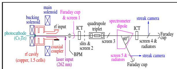
Figure 1: Schematic overview of PITZ 1. Beam direction is from left to right, and the total length is about 6 m.
