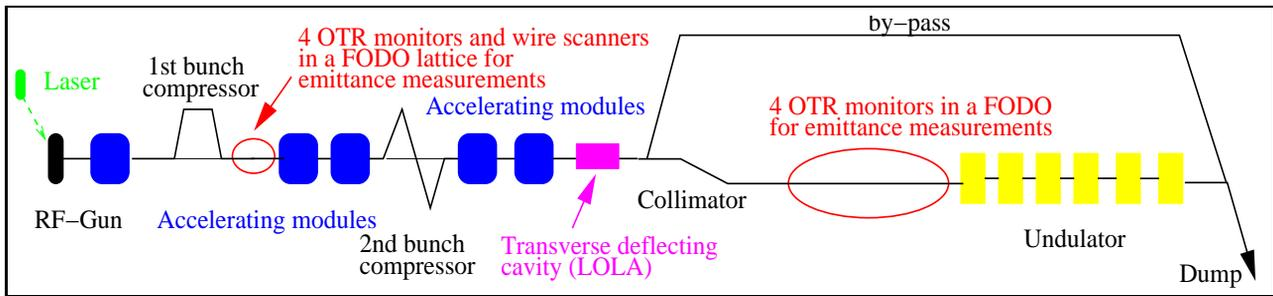
Figure 4: Present layout of the VUV-FEL linac (not to scale). Beam direction is from left to right. The total length is about 250 m. The LOLA cavity as well as the locations of the diagnostic sections dedicated to emittance measurements are indicated.
