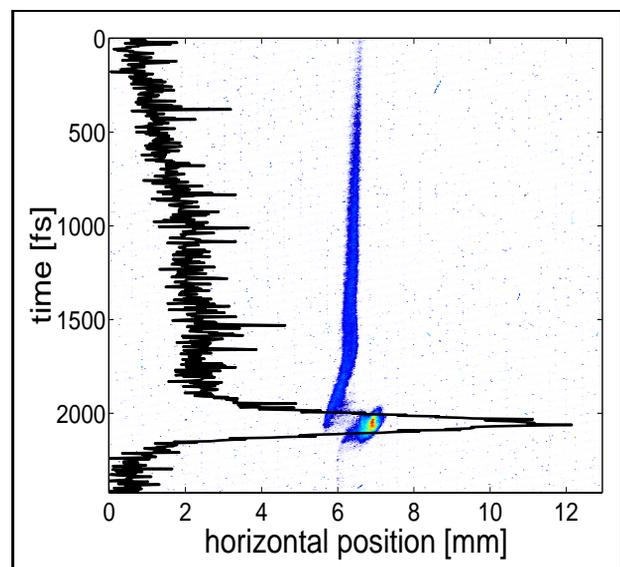
Figure 6: Longitudinal bunch distribution measured with the LOLA cavity during FEL operation.
