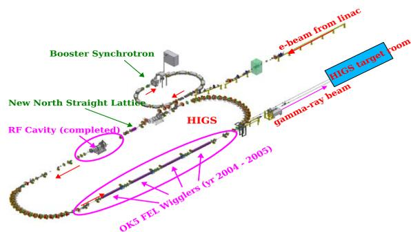
Figure 1: Fully upgraded Duke storage ring light source facility in 2006 with a HOM-damped RF cavity, a new 0.25 – 1.2 GeV booster, one new straight section to host FELs, and the other new straight for booster injection and future light sources.
