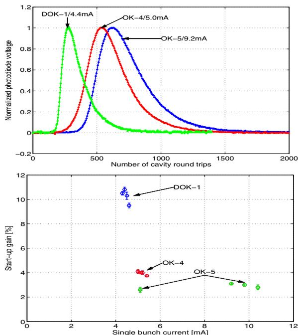
Figure 5: Measurements for the startup gain of the OK-4, OK-5, and DOK-1 FELs at 450 MeV. Upper plot: measured giant pulses produced by the three FELs with different currents; Lower plot: the start-up gain of the three FELs obtained by fitting the rise of the giant pulse to an exponential growth curve.
