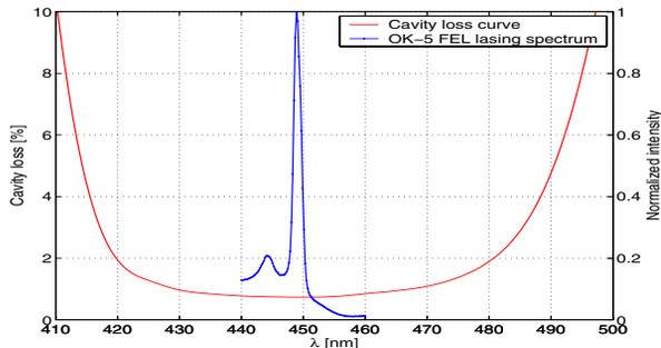
Figure 3: The first lasing spectrum of the OK-5 FEL with about 15 mA of single-bunch current at 274 MeV with a FWHM  $\Delta\lambda/\lambda = 3.4 \times 10^{-3}$ .
