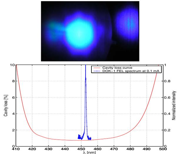
Figure 4: First demonstrations of DOK-1 FEL lasing at 450 MeV. Upper figure, the laser image on a diagnostics screen with the DOK-1 FEL lasing with 9.6 mA of single bunch current; Lower figure, the measured DOK-1 FEL spectrum with 0.1 mA of single bunch beam current.
