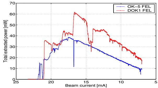
Figure 6: Measured total extracted power vs. the single bunch current for OK-5 and DOK-1 FELs at 450 MeV.
