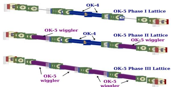
Figure 2: Three phases of the FEL upgrade project. The second phase allows the commissioning of the OK-5 FEL with two wigglers and DOK-1 FEL with two OK-4 and two OK-5 wigglers.
