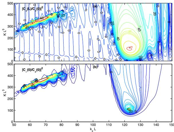
Figure 4: (a) Transmission and (b) reflection contours in the  $(k_z L, \kappa L^3)$  plane for free-electron laser. Logarithmic scale in [dB].
