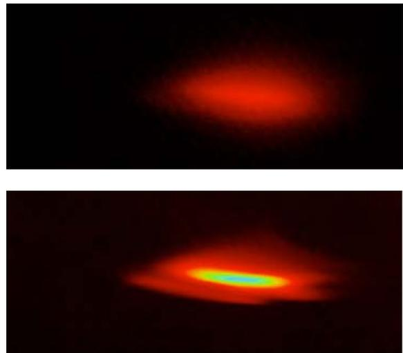
Figure 3. Electron beam imaging using Cr-oxide (top) and Ce-doped YAG radiators (bottom). Electronic gain of the CCD camera was approximately three times higher in the case of Cr-oxide screen to get comparable pixel values with the Ce:YAG.
