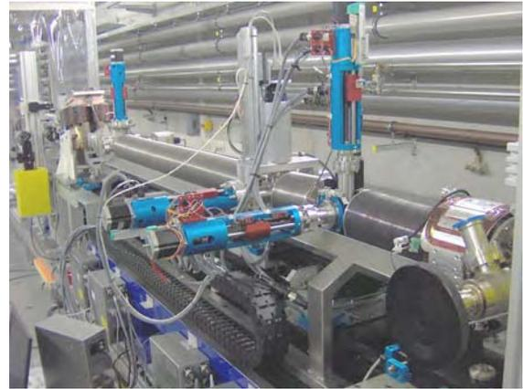
Figure 5. SPARC e-meter during installation at the Photo Injector Test Facility PITZ.
