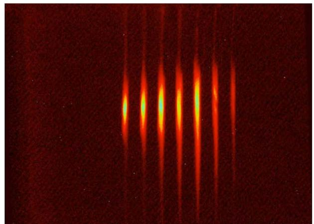
Figure 6: Picture of the beam at the YAG screen downstream the multi-slit mask.
