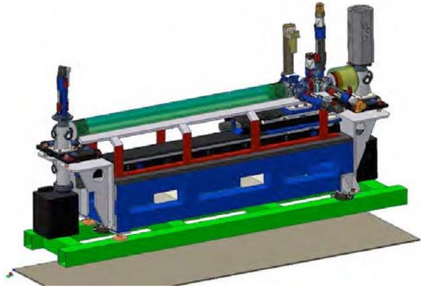
Figure 1. 3D mechanical drawing of the SPARC e-meter. In this drawing are also included one of the two alignment tools, to be installed during alignment on top of the end flanges (grey cylinders), and the PITZ girder (green structure).
