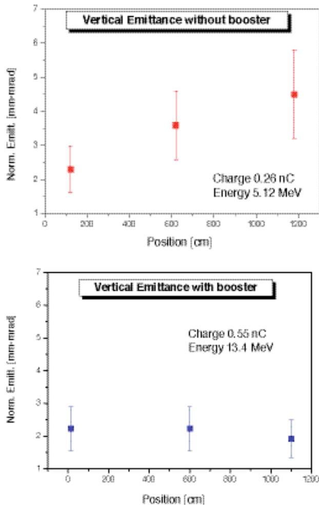
Figure 7: Preliminary result of vertical emittance measurements at PITZ with the SPARC e-meter under different conditions (booster off/on). Note that the three z-positions are not coincident in the two cases; also the beam charge is not identical.
