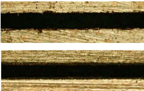
Figure 2. Optical microscope pictures of the single-slit obtained by mechanical machining (top) compared to single-slit produced by photo-chemical machining (bottom).
