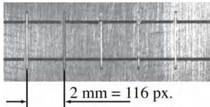
Figure 4. On-line measurement of resolution of the optical system can be done using the calibration marks on the screen holder.
