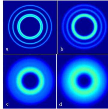
Figure 6: Expected diffraction patterns of electrons with different divergences of 0.05 (a), 0.1 (b), 0.2 (c), and 0.3 (d) mrad.
