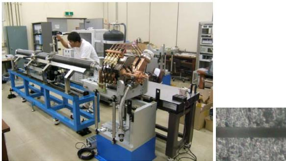
Figure 1: Appearance of emittance meter (left). Right figure is magnified view of 40-μm width slit mode on 0.5-mm thick tungsten plate.
