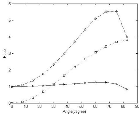
Figure 5: Quantum efficiency (top), R, and reflectivity changes vs. incidence angle of p-polarized photons.
