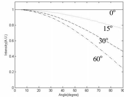
Figure 3: Angular distributions of photoelectrons for different incidence angle of p-polarized photons.
