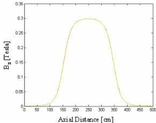
Figure 9: Measured on-axis B<sub>z</sub> profile. Excitation current was 200 A. Field uniformity at magnet center is ~10<sup>-4</sup>. Offset between mechanical and field centers are approximately 0.1 mm.
