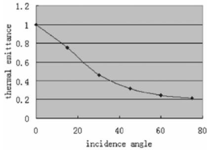
Figure 4: Cathode intrinsic emittance of photoelectrons by p-polarized photons at oblique incidence.
