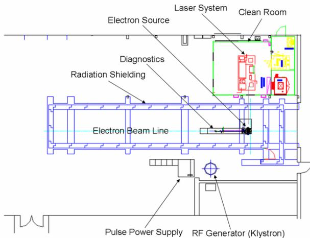
Figure 7: Layout of GTS (Gun Test-Stand) at the PAL.
