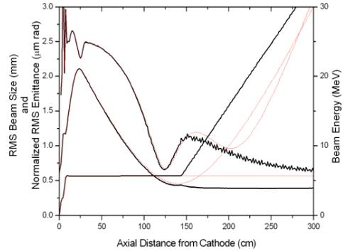
Figure 2: PARMELA simulation of emittance and beam size profiles for LCLS-style injector. Thin (red) lines are for those without acceleration. Thick (black) ones are for those with acceleration.
