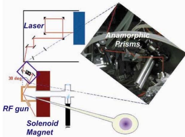
Figure 3: Top view of the slanting injection method with the anamorphic prisms.
