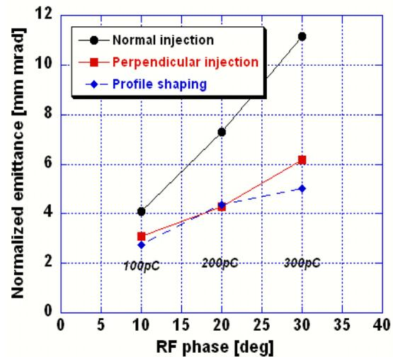
Figure 6: Minimum normalized emittance of each injection method as a function of rf phase
