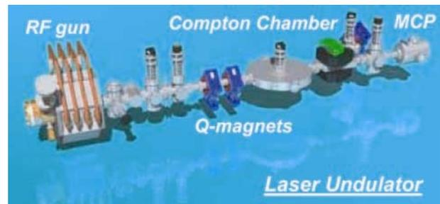
Figure 1: Laser Undulator as a compact soft X-ray source
