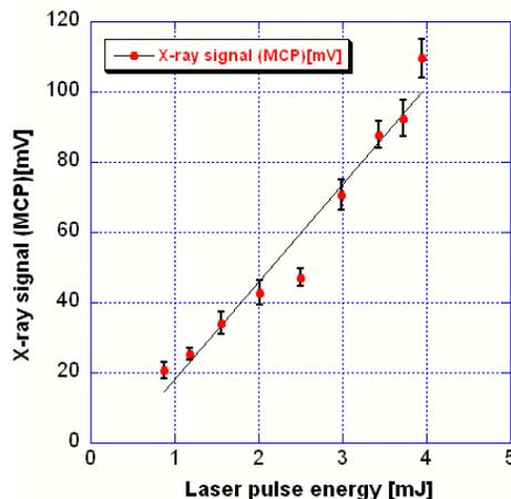
Figure 2: the typical soft X-ray signals as a function of the laser energy
