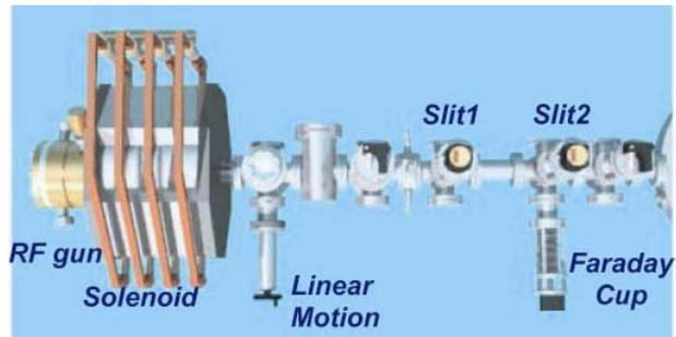
Figure 4: Top view of the experimental setup on the emittance measurement.
