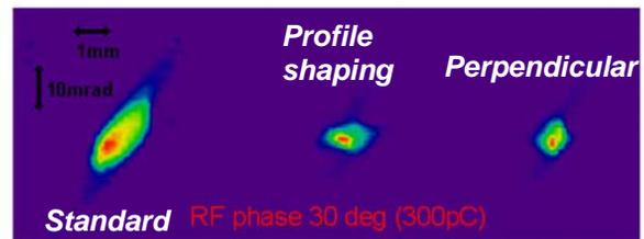
Figure 5: the minimum emittance distributions of the electron beam at 30 degree rf phase corresponding to charge of 300 pC .
